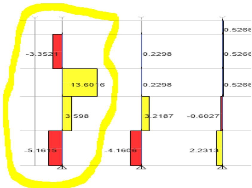
Figure 6 -Shear for column design.
